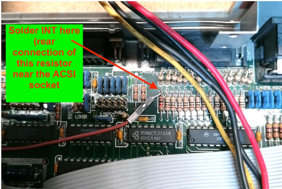
You should remove the VME metal cage before. The soldering point is located underneath and is not easy to reach otherwise.
