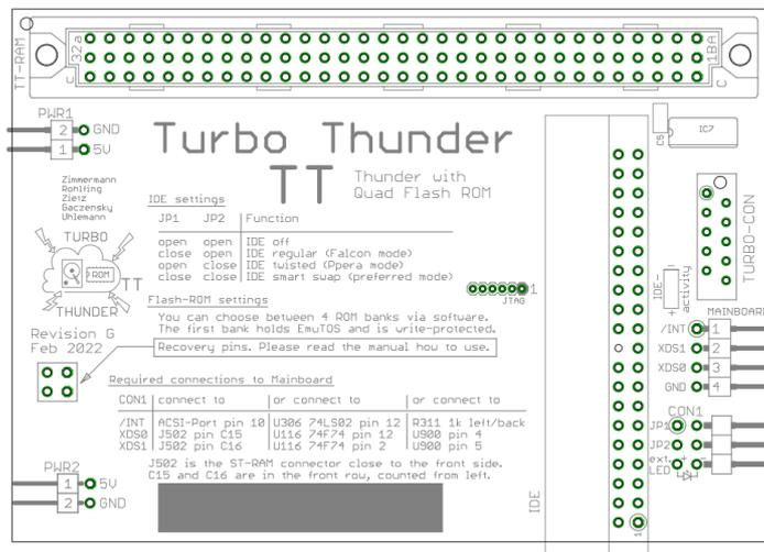
On the right side of the PCB you will find three connectors. In top the connector side the "Turbo-CON" - reserved for future features. In the middle the connector is for the three required connections to the mainboard: /INT, XDS0 and XDS1. The jumper block "CON1" which gives you to opportunity to define the operation mode of IDE and the option of connecting a second IDE activity LED.
