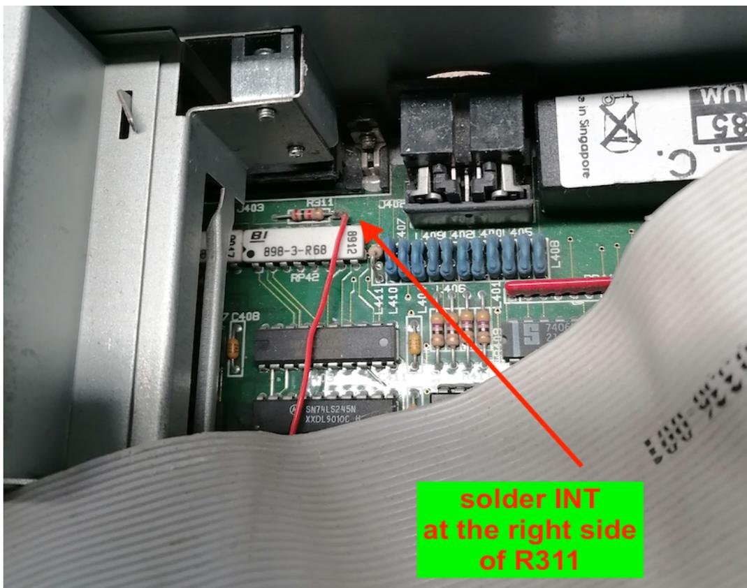
With a little skill you can lay the cable under the VME metal cage. You will find R311 at the rear edge next to the external floppy socket. In case B this location is reasonably easy to access.
